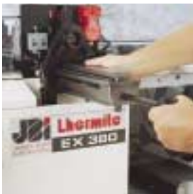
Heavy duty tempered steel die changes are quick and easy on all three models.
